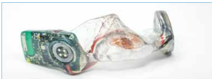
Fig. 2: Wireless oral device to control the piano pedals
